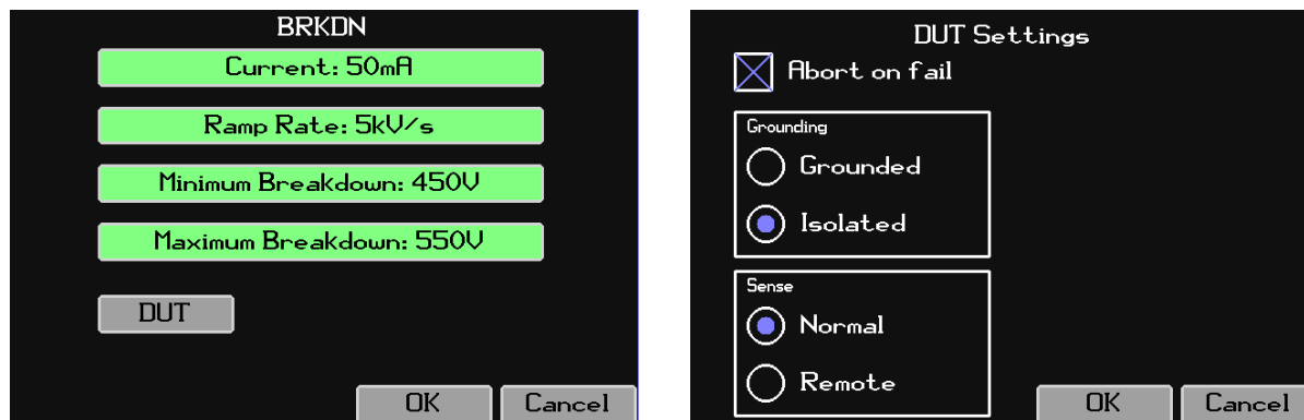
Figure 7-25 BRKDN Step Configuration Screens
