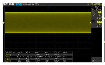
SDS1004X-U can measure all sampled data points up to 14 Mpts. This ensures the accuracy of measurements while the math co-processor decreases measurement time and increases ease-of-use.
