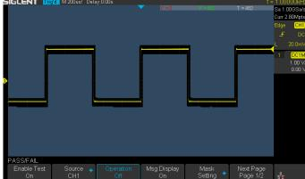
The SDS1000X-U utilizes a hardware-based Pass/Fail function, performing up to 40,000 Pass / Fail decisions each second. Easily generate user defined test templates provide trace mask comparison making it suitable for long-term signal monitoring or automated production line testing.
