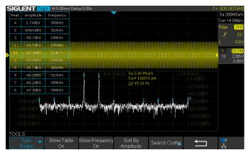
The math co-processor enables FFT analysis of incoming signals using up to 128k samples per waveform. This provides high frequency resolution with a fast refresh rate. The FFT function also supports a variety of window functions so that it can adapt to different spectrum measurement needs. It also supports Peaks, Markers, a variety of numbers.
