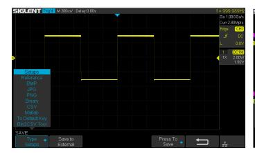
The current parameters of the oscilloscope can be preset to Default Key through the Save menu.
