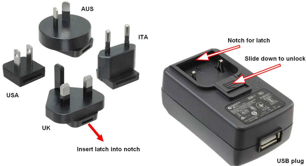
Fig. 10-11 AC/DC Power Supply / battery charger
