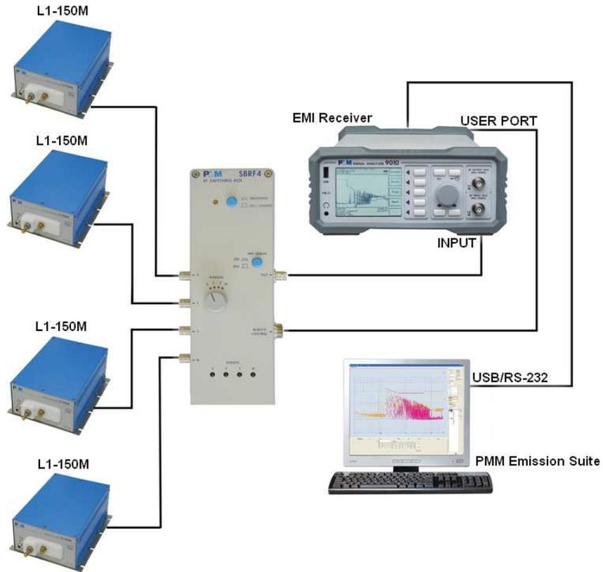
**Fig. 8-5** PMM SBRF4 with external Artificial Mains Network
