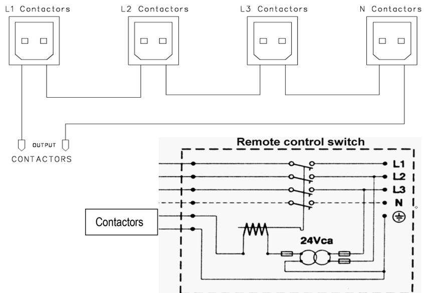
**Fig. 5-5 Contactors diagram**
