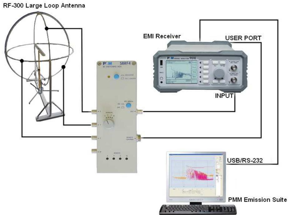
**Fig. 8-6** PMM SBRF4 with RF300 Large Loop Antenna
