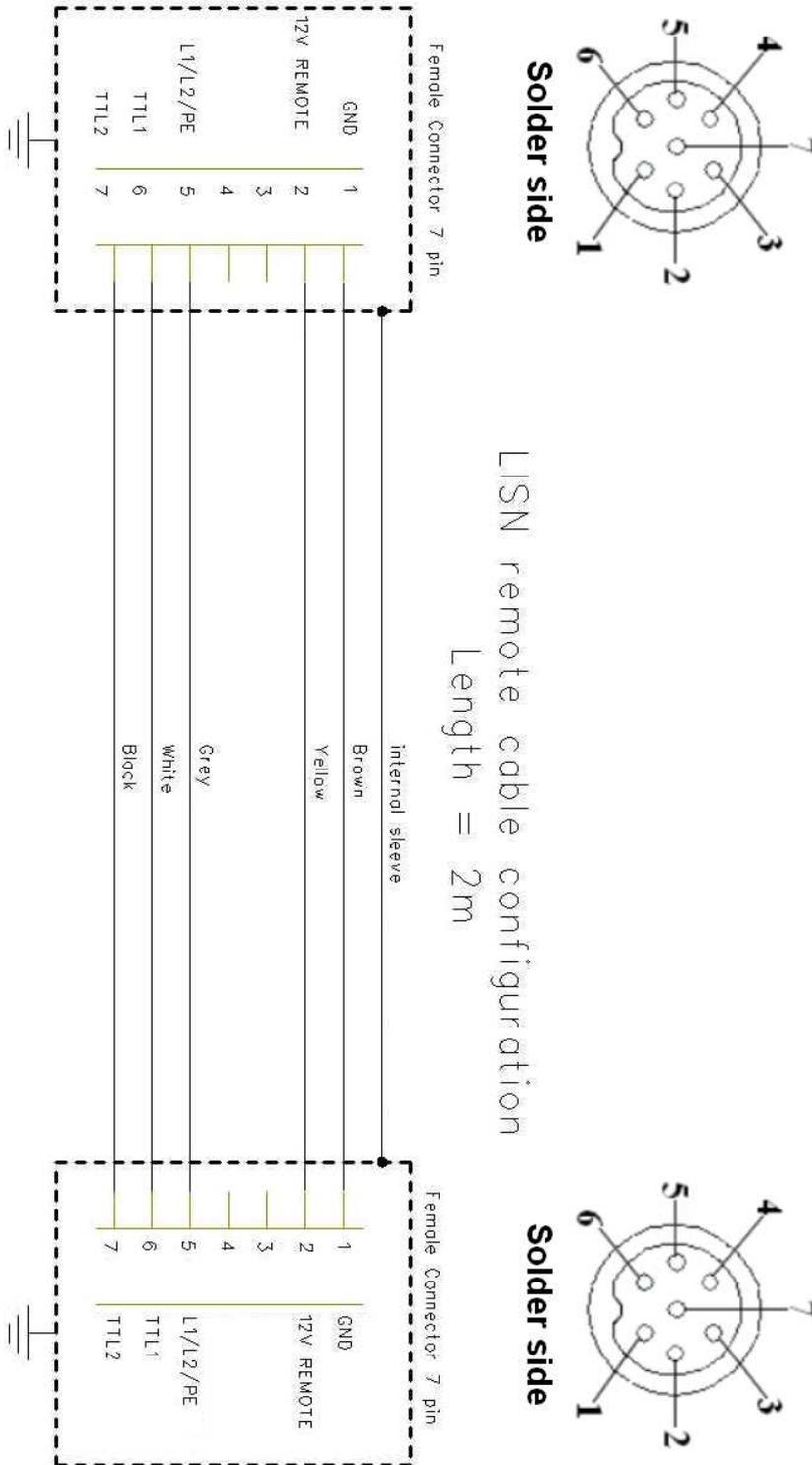
**Fig. 7-4 LISN remote cable configuration for PMM 8010**
